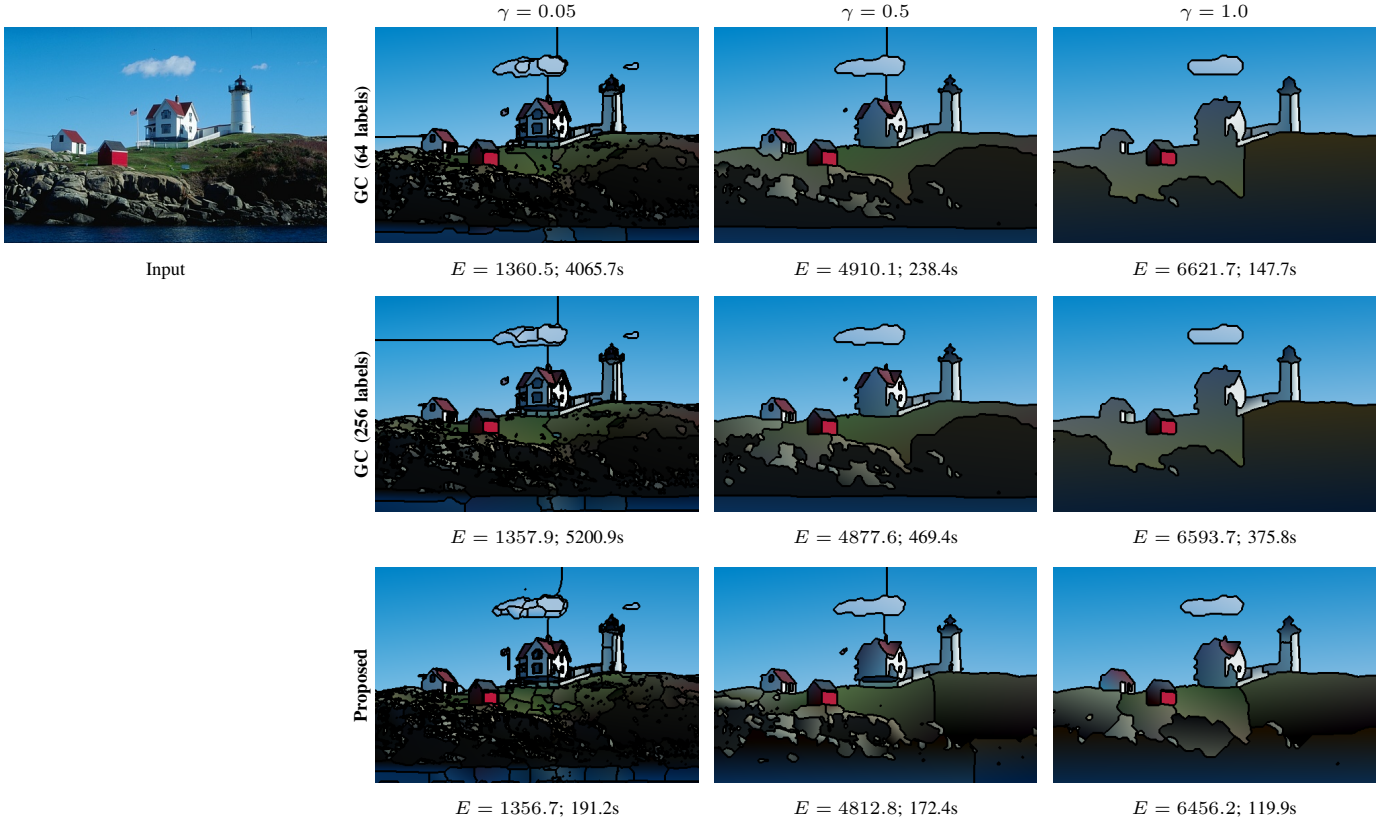
Fig. 4: Qualitative comparison to graph cuts. The proposed approach and the graph cut approach both provide reasonable partitions yet with some slight differences. For example at \gamma = 0.5 , graph cuts still opens a segment for the water, but not for the fence. In the proposed approach, this is vice versa. As a general tendency, we observe that the proposed approach results in more segments throughout all \gamma -levels.
