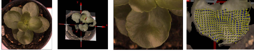
Fig. 7.18. reconstruction of plant using 49 camera positions. From left to right: central image of input sequence, rendered depth estimates, close-up view on leaf and estimated depth with surface slopes
