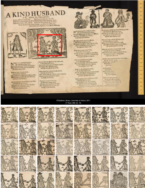
Figure 2: The upper image shows the query region marked with a rectangle. The lower image shows the first 40 responses for this search run. It can be seen that the lower rows show detections which have some variability to the query object. In the last row, there are the first wrong detections.
