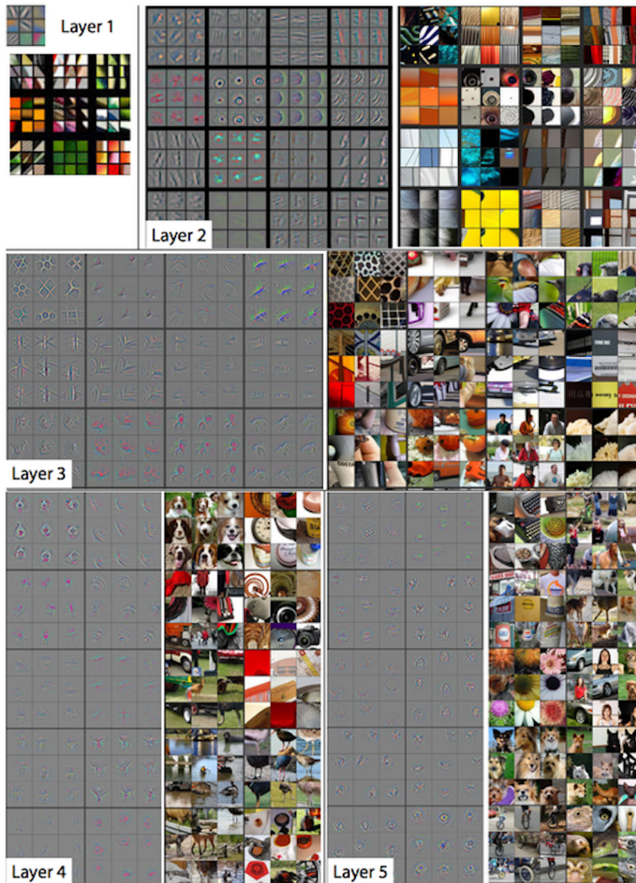
Figure 2: Visualization of the kernels (grey) and features (images) of a VGG network trained to classify the 1000 classes of the IMAGE-Net dataset. The complexity of the features the CNN extracts increases hierarchical for every layer. It becomes apparent especially for the higher level features, that the features are useful to detect humans, animals, cars etc. which are a subgroup of the 1000 classes. The network learns to detect useful features for the classification task by itself.
